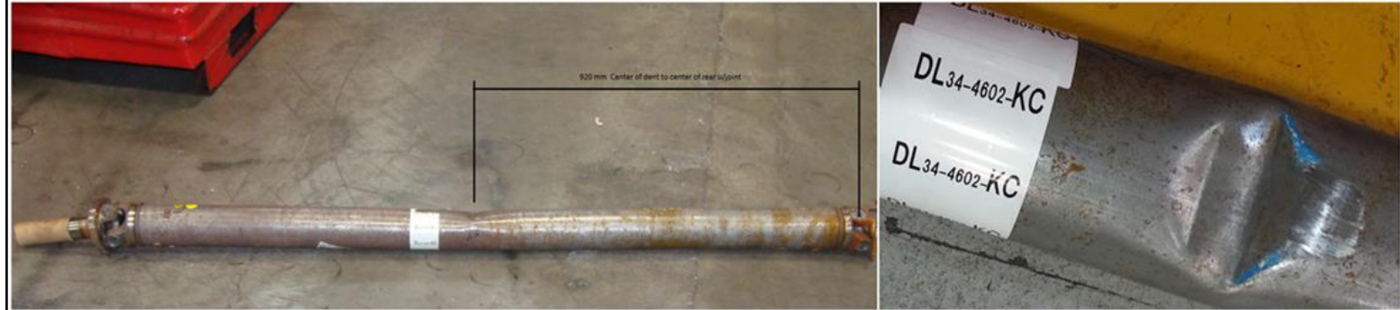
2-Pc Shipping Damage "Axle Shaft"
