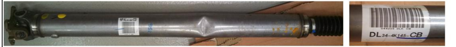
2-Pc Shipping Damage "Axle Shaft"
